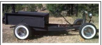
1932 Ford pickup rolling chassis includes: pickup bed; four 15" chrome reverse wheels; original 'K' member and cross members; front fender braces; radiator; headlight bar; and steering box and column with original key in column lock. The torque tube and rear end were chromed in the 1960's Price: \$3500
